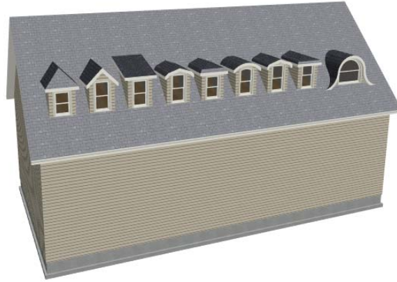
Hip, Gable, Shed, Gambrel, Mansard, Barrel, Curved Eave, Hip Curved Eave, and Eyebrow dormer roof types
